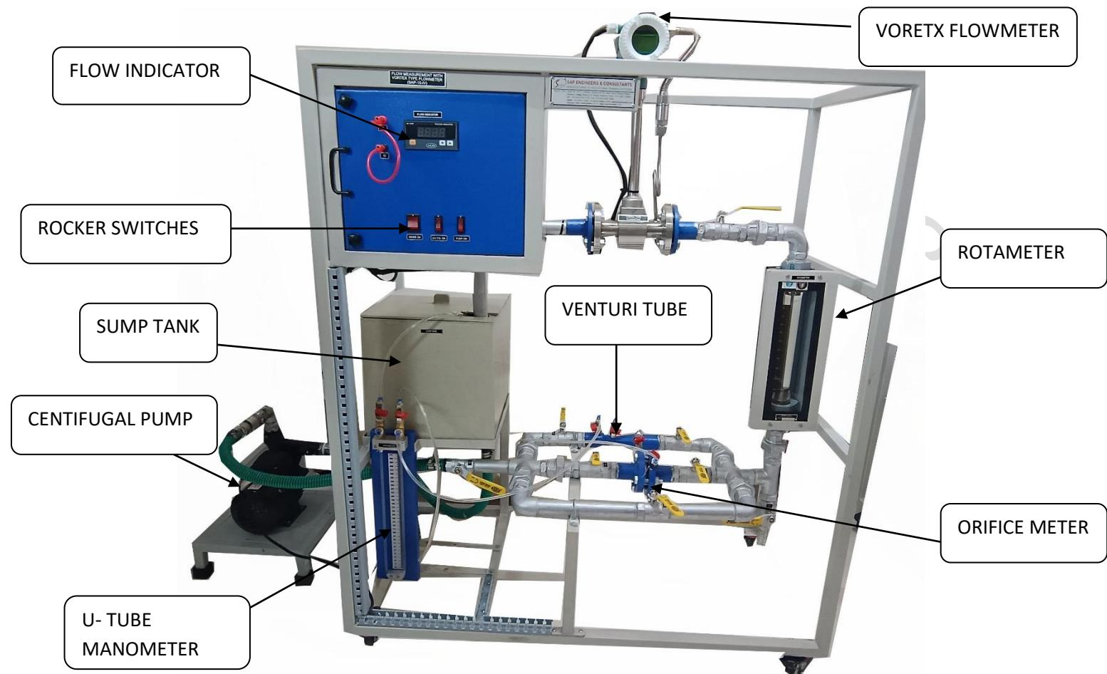
The **Setup for Calibration of Flow Sensor (SAP – 15D-IV)** gives an idea regarding Flow Sensor & Flow Transmitter Principle. It outlines the procedure for calibration of flow Sensors/Transmitters.
